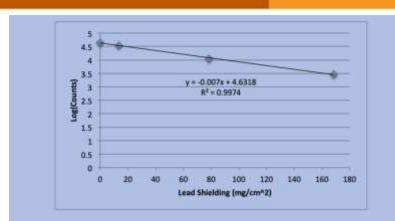
Figure 3: Logarithmic relation between shielding and gamma counts, discounting data points where final range of linearity and penetration was reached.
